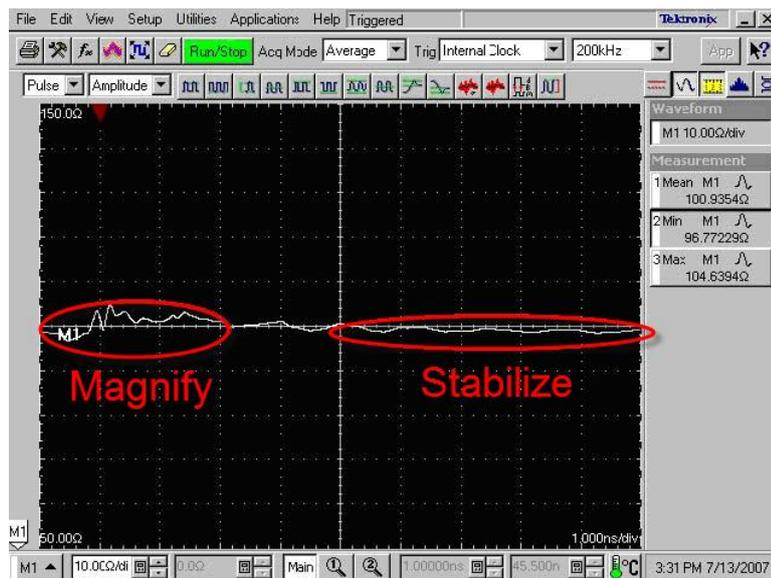
Figure 29 Waveform Stabilizes
