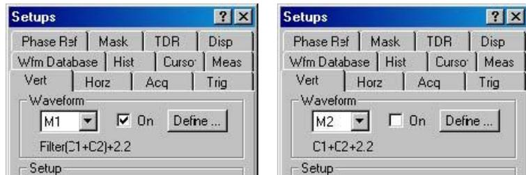
Figure 28 Setting filtered M1 to ON, unfiltered M2 to OFF
