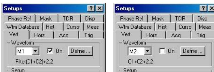
Figure 19 Setting filtered M1 to ON, unfiltered M2 to OFF
