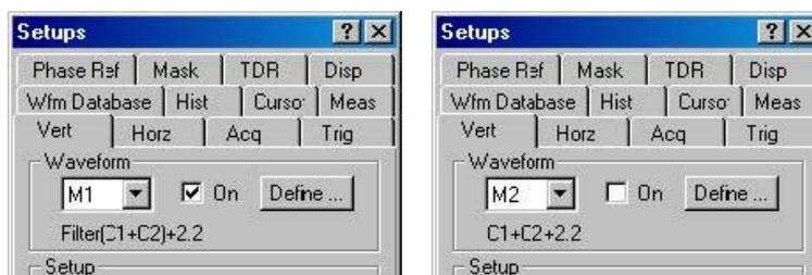
Figure 22 Setting filtered M1 to ON, unfiltered M2 to OFF
