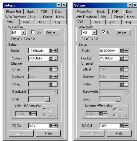
Figure 15 Setting filtered M1 to OFF, unfiltered M2 to ON
